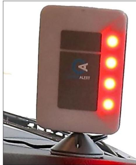
*The cab unit flashes an alert and emits an audible alarm to warn the driver of a nearby cyclist, and also illuminates several LED lights to indicate that bicycle's location relative to the vehicle.*
